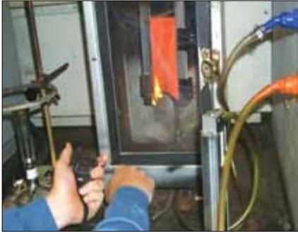
Fig. 1: The ASTM D6413 vertical flame test.
