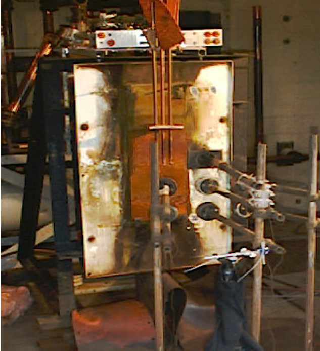
FIGURE 3. Test Setup No. 2 3-Phase Flat Electrodes in Front of Plane
